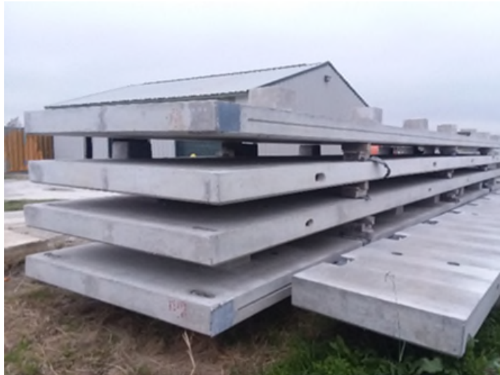
Typical Spandrel Panels in Storage
